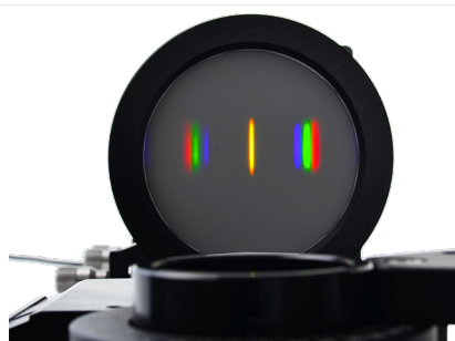
Fig. 4.45: Spectral distribution of the white LED seen behind the grating
