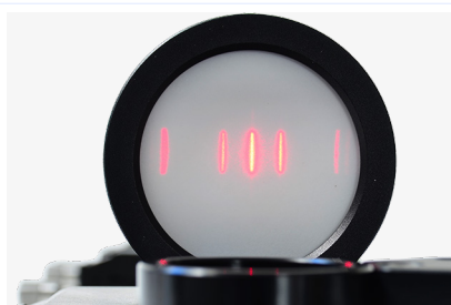
Fig. 4.47: Spectral distribution of the laser diode
